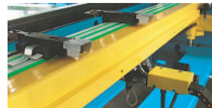
Back gauge mod. RPL with 4 axes (X Z1 Z2) with movement of back gauge fingers controlled by CNC.
